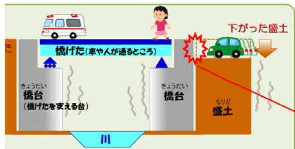
Fig.2 A step after an earthquake
